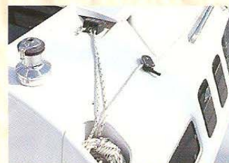
All lines are led aft for short-handed sailing and the coaming wells keep it all organized.
