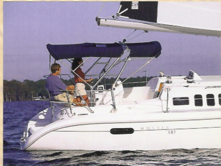
The integrated arch keeps the cockpit clear with the traveler up top and makes a great attachment point for the optional bimini.
