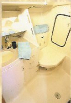
The covered marine head doubles as a shower seat in the enlarged head. Corian® counters and plenty of dry storage is a must.
