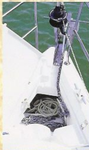
The stainless steel anchor roller leads into a deep well that can handle all the chain and rode you need.
