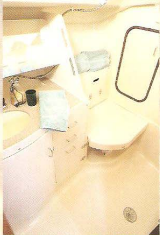
The covered marine head doubles as a shower seat in the enlarged head. Corian® counters and plenty of dry storage is a must.
