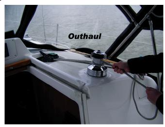
Turn into the wind. Release clutches on both the furling line and outhaul. Simultaneously pull on outhaul while unfurling with the left side blue furling line. Engage clutches when finished.
